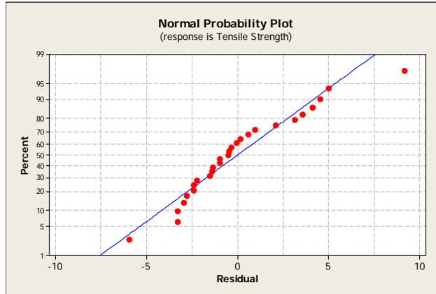
**Fig. 7.** Normal probability of the residuals for Tensile strength
