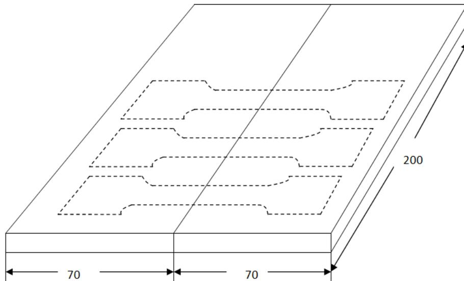
Fig. 3. Schematic view of the FS Welded Joint with the extraction of tensile specimens
