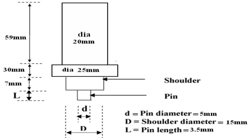
Fig. 2 Geometry of the rotating tool
