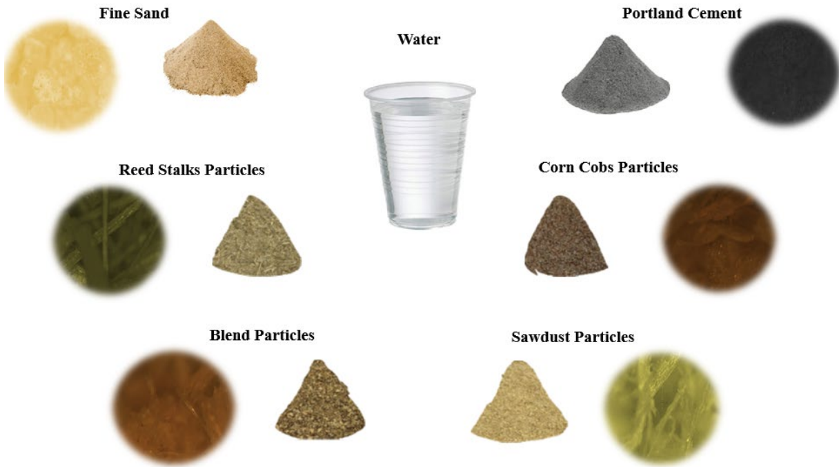
Fig. 2. The blend of individual particles for mortar under the microscope, including Insulated Material, Portland Cement, Fine Sand, and Water.
