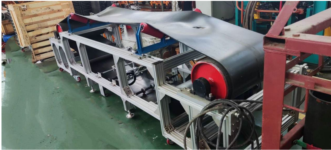
Fig. 1. Conveyor belt test platform physical picture
