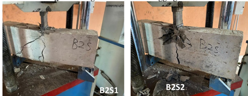
Fig. 7. Damage mode of 25 mm aggregate beam
