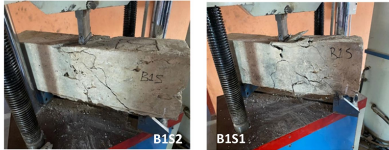
Fig. 6. Damage mode of 50 mm aggregate beam
