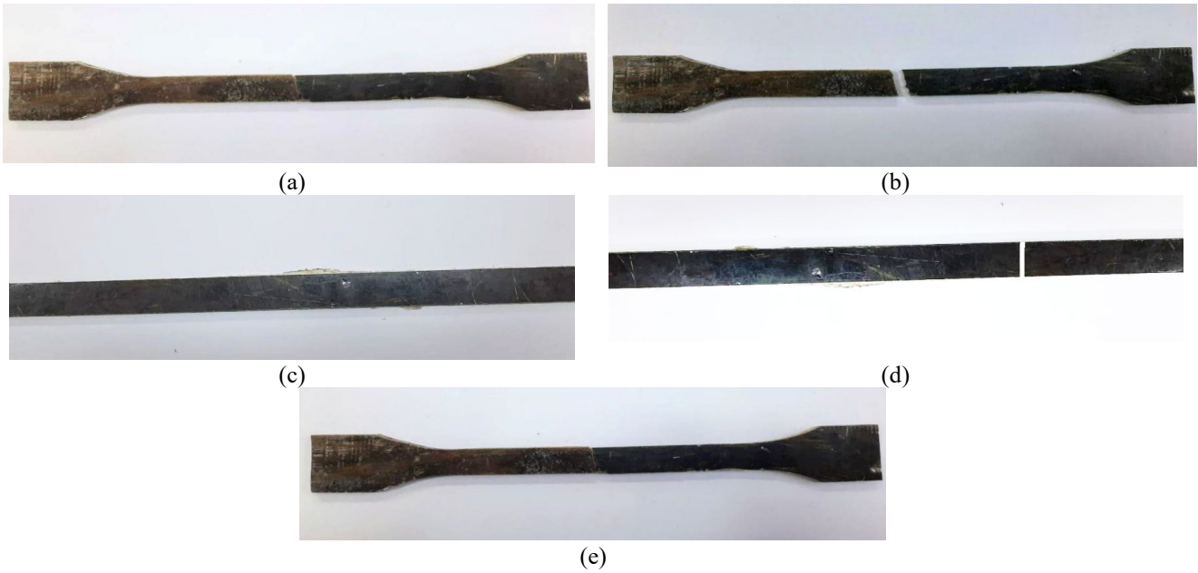
Fig. 6. (a) to (e) Images of some experimental testing kenaf-coir-based hybrid composite incorporated with titanium carbide nano-fillers samples for mechanical testing.
