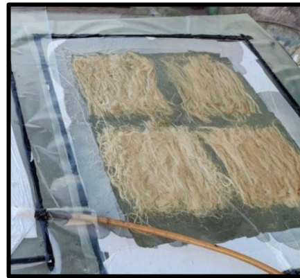
Fig. 4. Samples placed on the sheet for Vacuum Bag Molding Process
