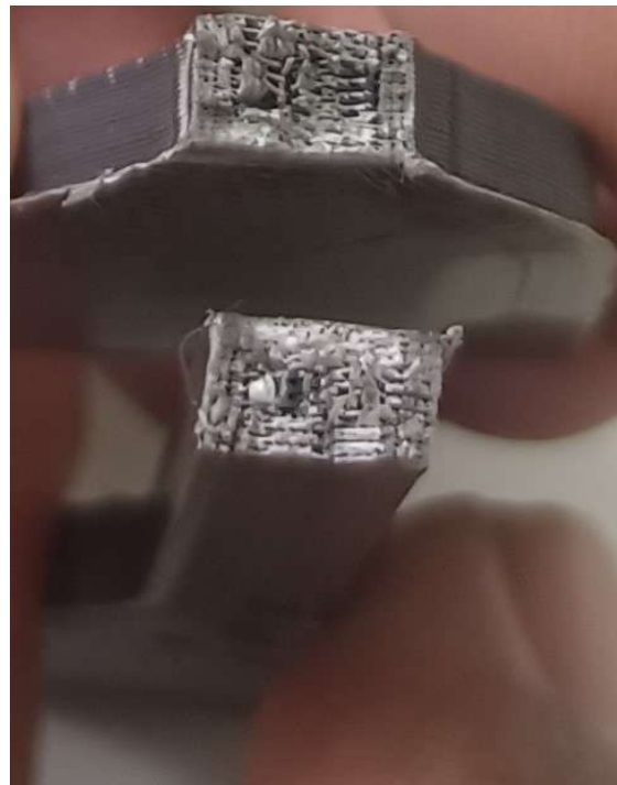
Fig. 6(b). Fractured surface of tensile test specimen
