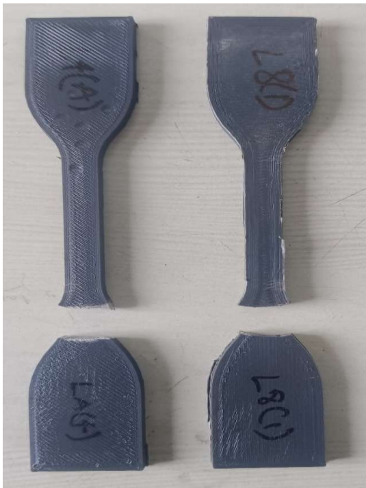
Fig. 6(a). Fractured tensile test specimens
