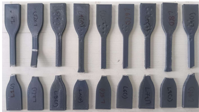
Fig. 5. Tensile test specimens after conducting tensile test on UTM.
