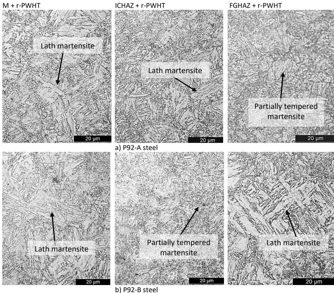
**Fig. 14.** Optical image of the as-received, ICHAZ, and FGHAZ after r-PWHT.
