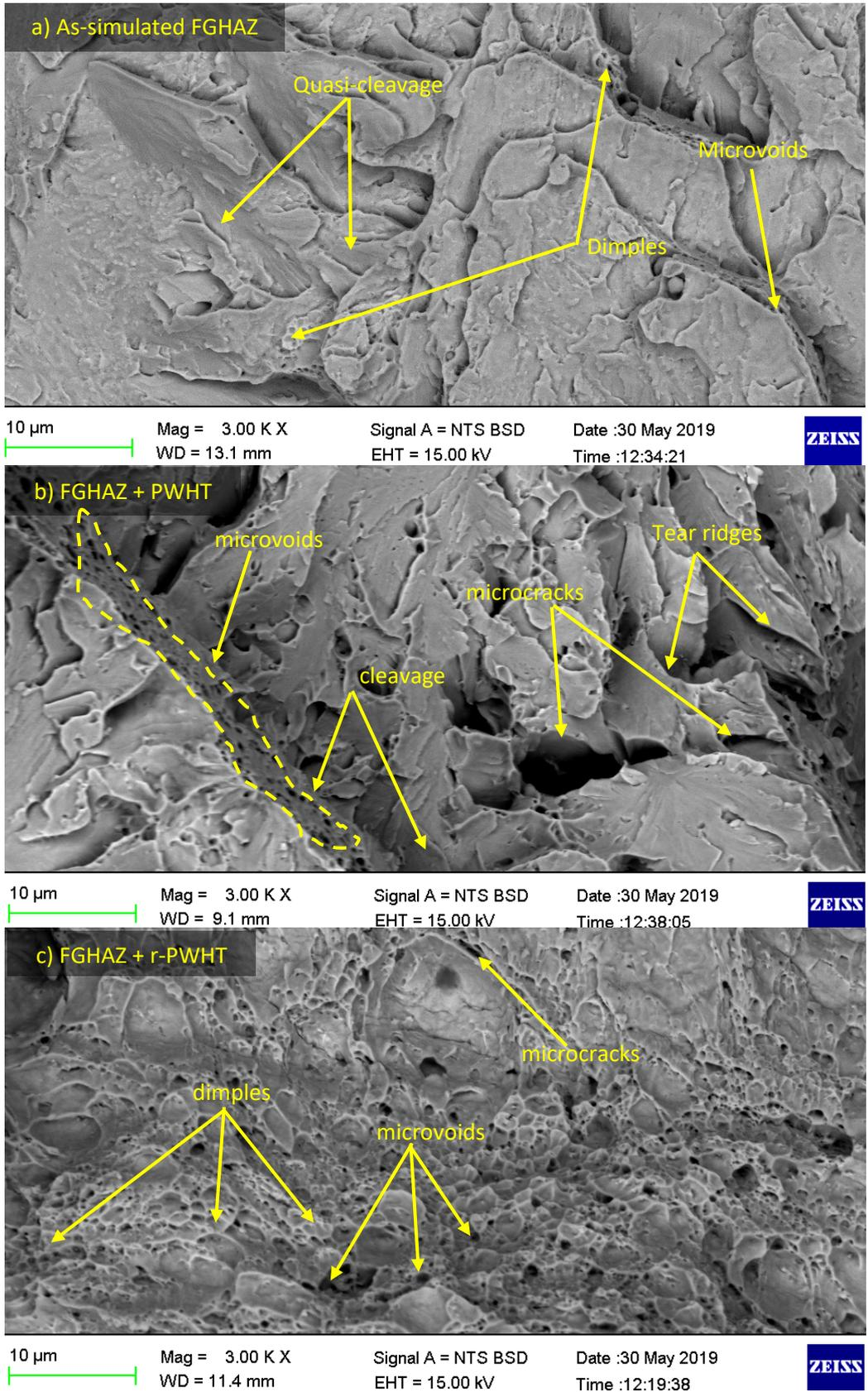
**Fig. 25.** SEM-BSE fractography image a) as-simulated, b) PWHT, and c) r-PWHT for P92-B steel.
