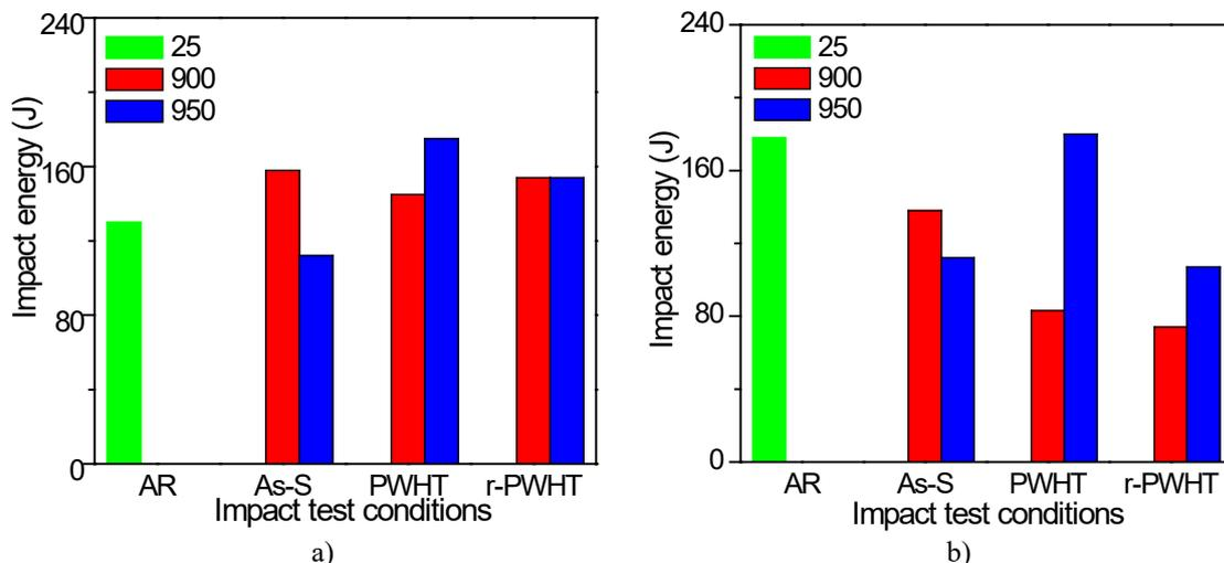
**Fig. 19.** Charpy toughness values at different processing conditions: a) P92-A and b) P92-B.
