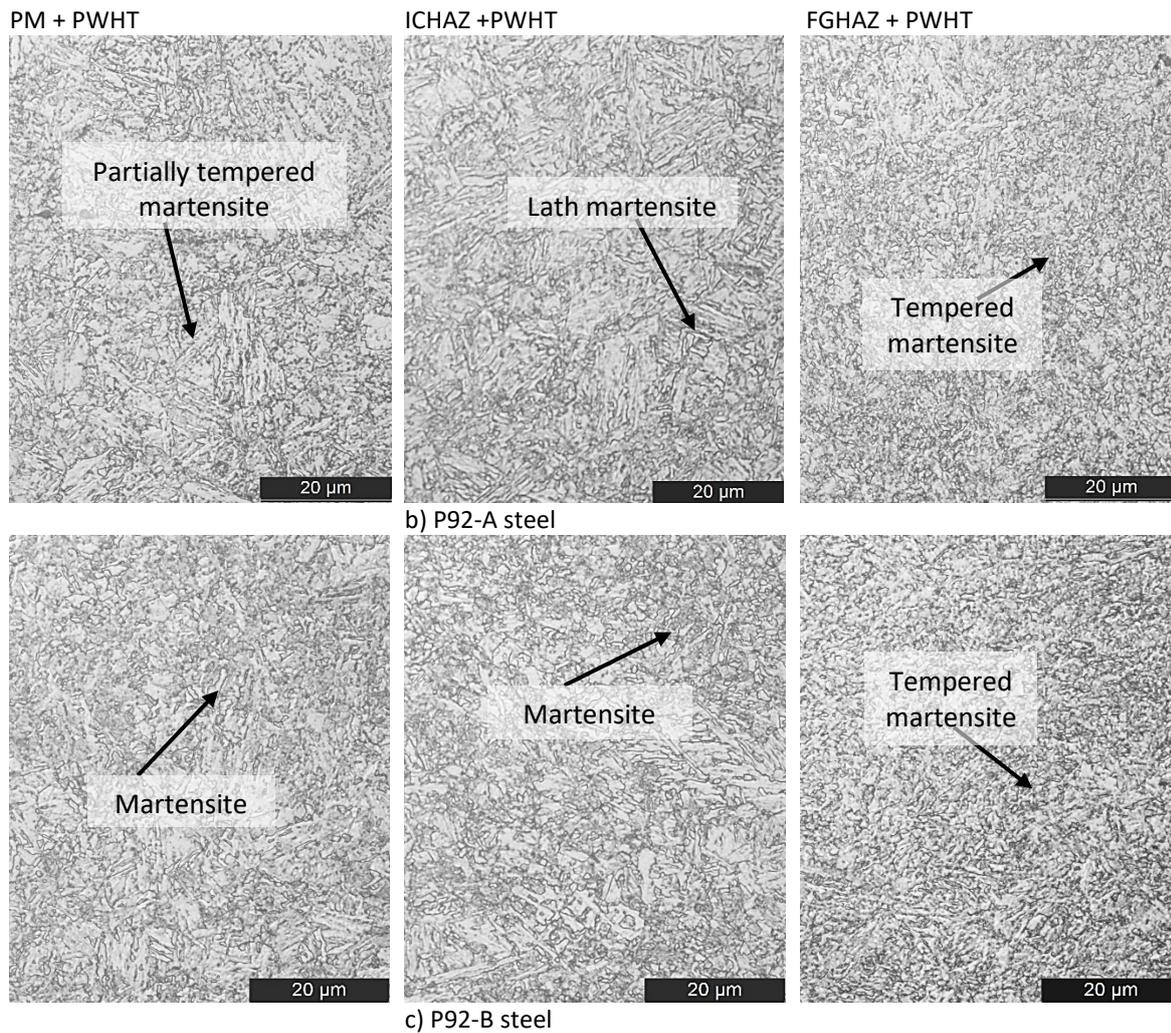
**Fig. 11.** Optical image of the as-received, ICHAZ and FGHAZ after PWHT for the two P92 steels.
