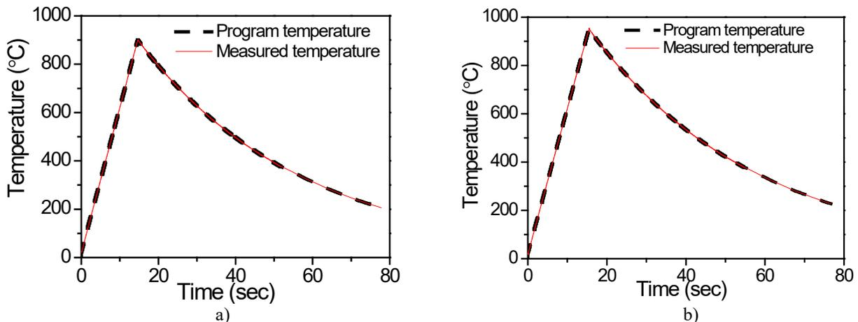
Fig. 4. Thermal cycle for HAZ microstructure simulation using the Gleeble® 3500 thermo-mechanical simulator a) 900 °C, and b) 950 °C.
