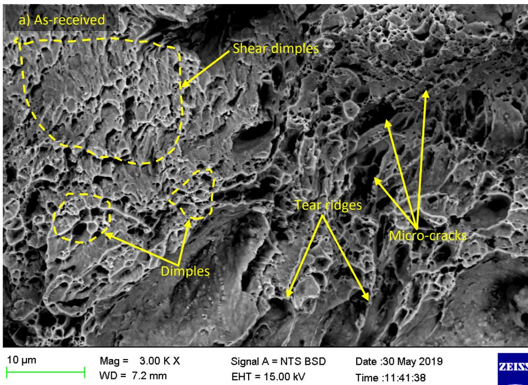
**Fig. 20.** SEM-BSE fractography image for P92-B steel.
