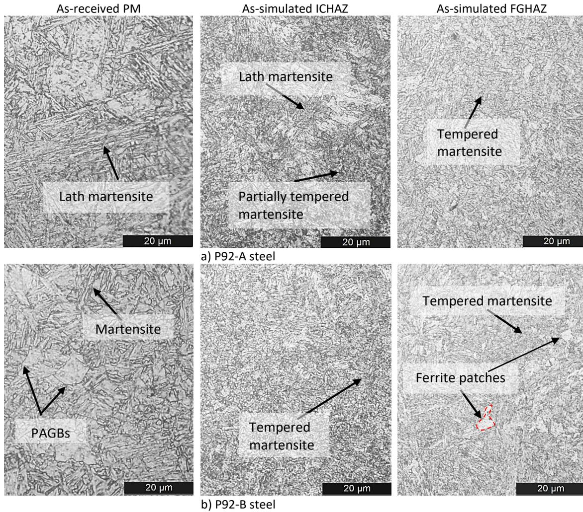
**Fig. 8.** Optical image of as-received parent metal and as-simulated HAZ microstructure.
