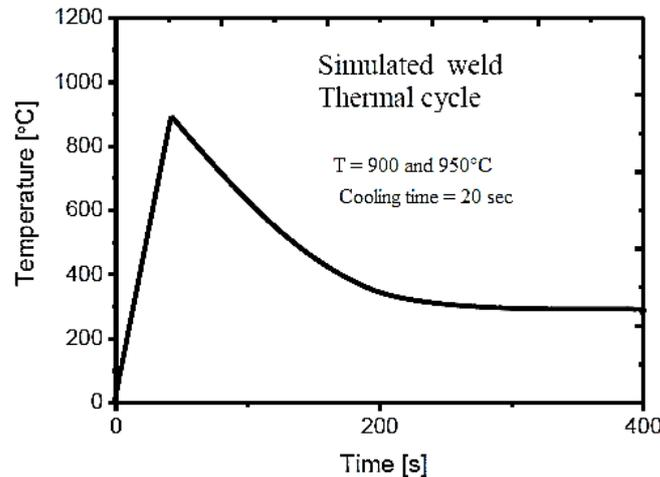
**Fig. 2.** Thermal cycle of weld joint simulation.
