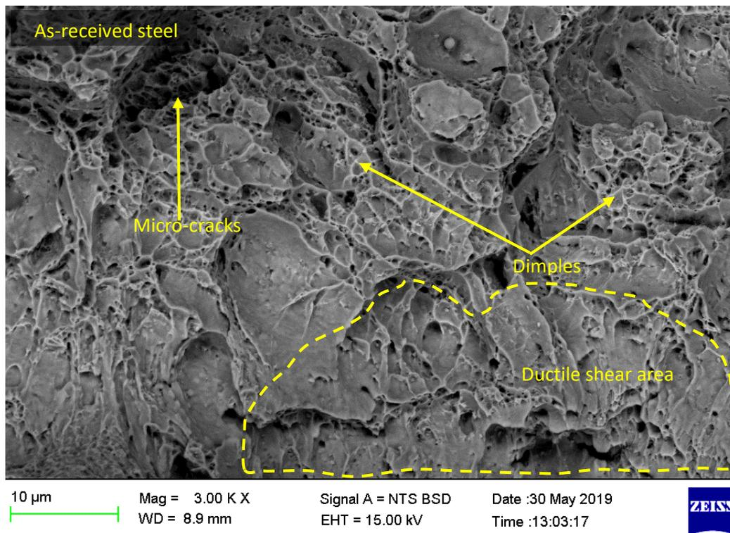
**Fig. 23.** SEM-BSE fractography image as-received P92-B steel.
