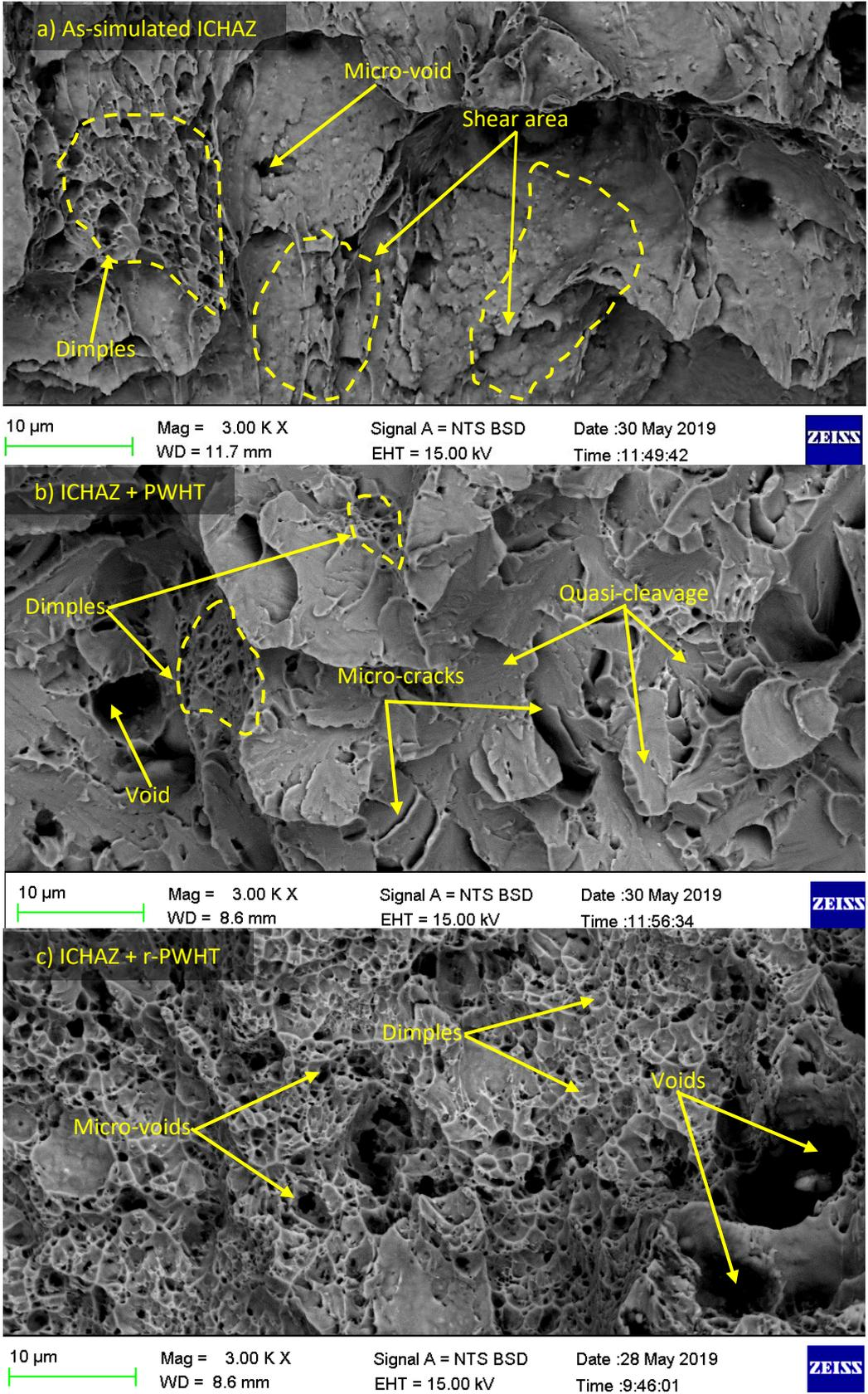
Fig. 21. SEM-BSE fractography image: a) PWHT and b) r-PWHT for P92-A steel.
