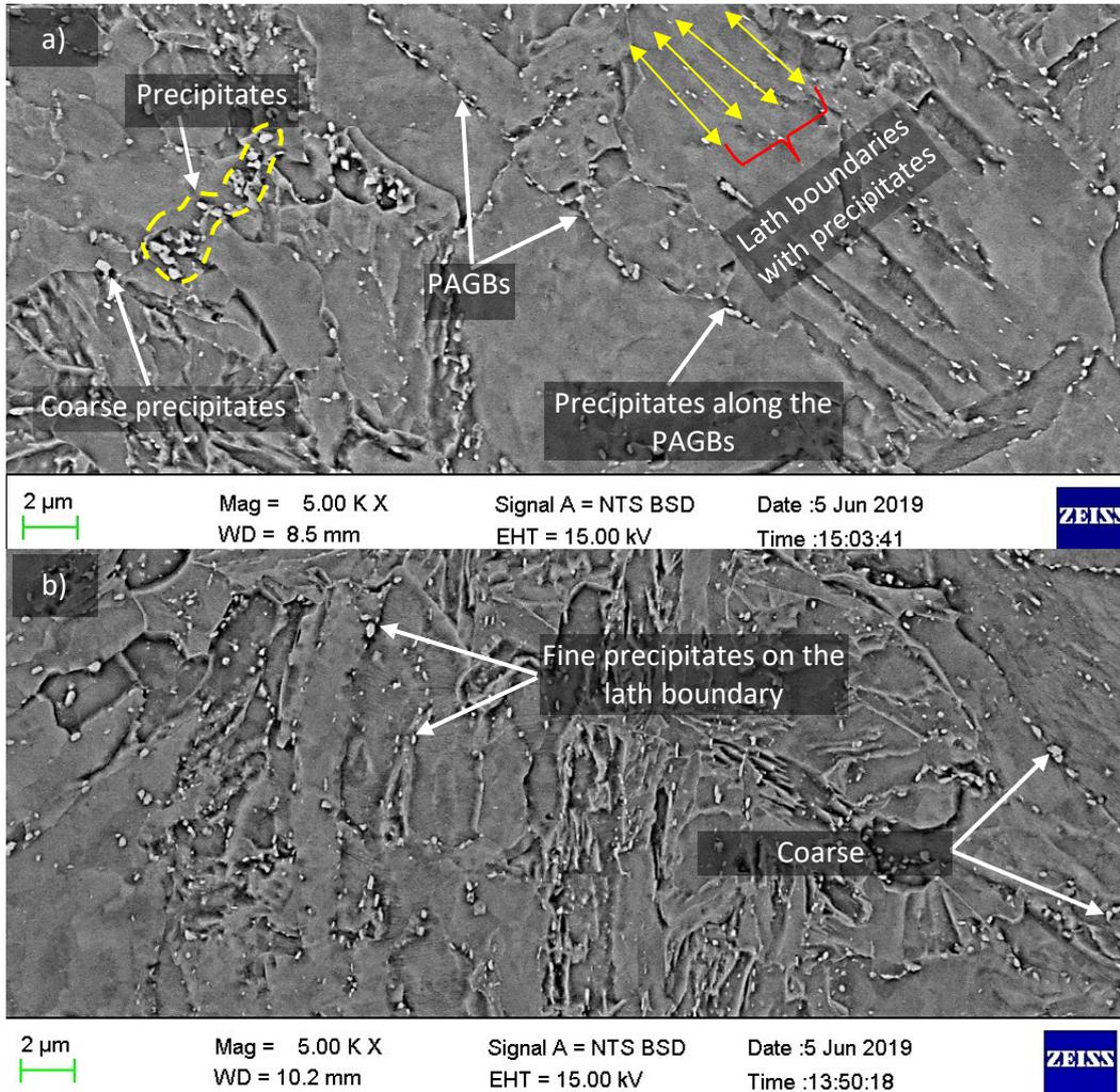
**Fig. 12.** SEM-BSE image of ICHAZ after PWHT a) P92-A b) P92-B.
