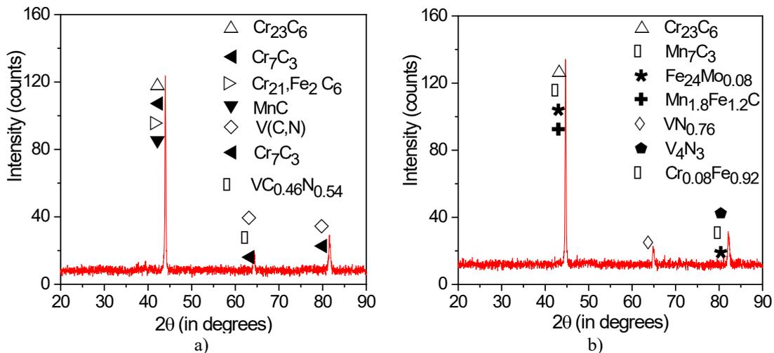
Fig. 7. XRD pattern for as-received base metals a) P92-A, b) P92-B.
