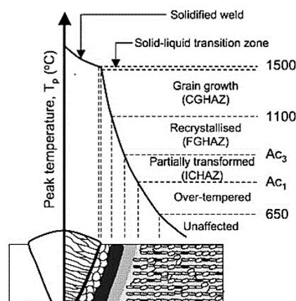
**Fig. 1.** An illustration of HAZ regions at various peak temperatures (Francis *et al.*, 2006).
