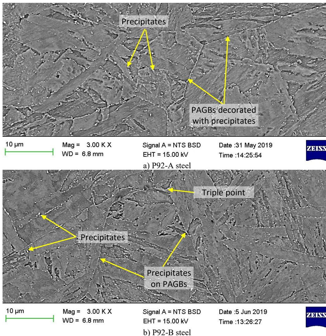
**Fig. 5.** SEM-BSE micrographs of as-received P92 steels.
