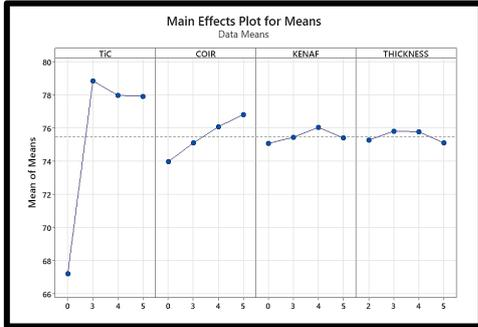
Fig. 8. Main effects plot of Tensile Strength for TiC reinforced kenaf coir hybrid composite
