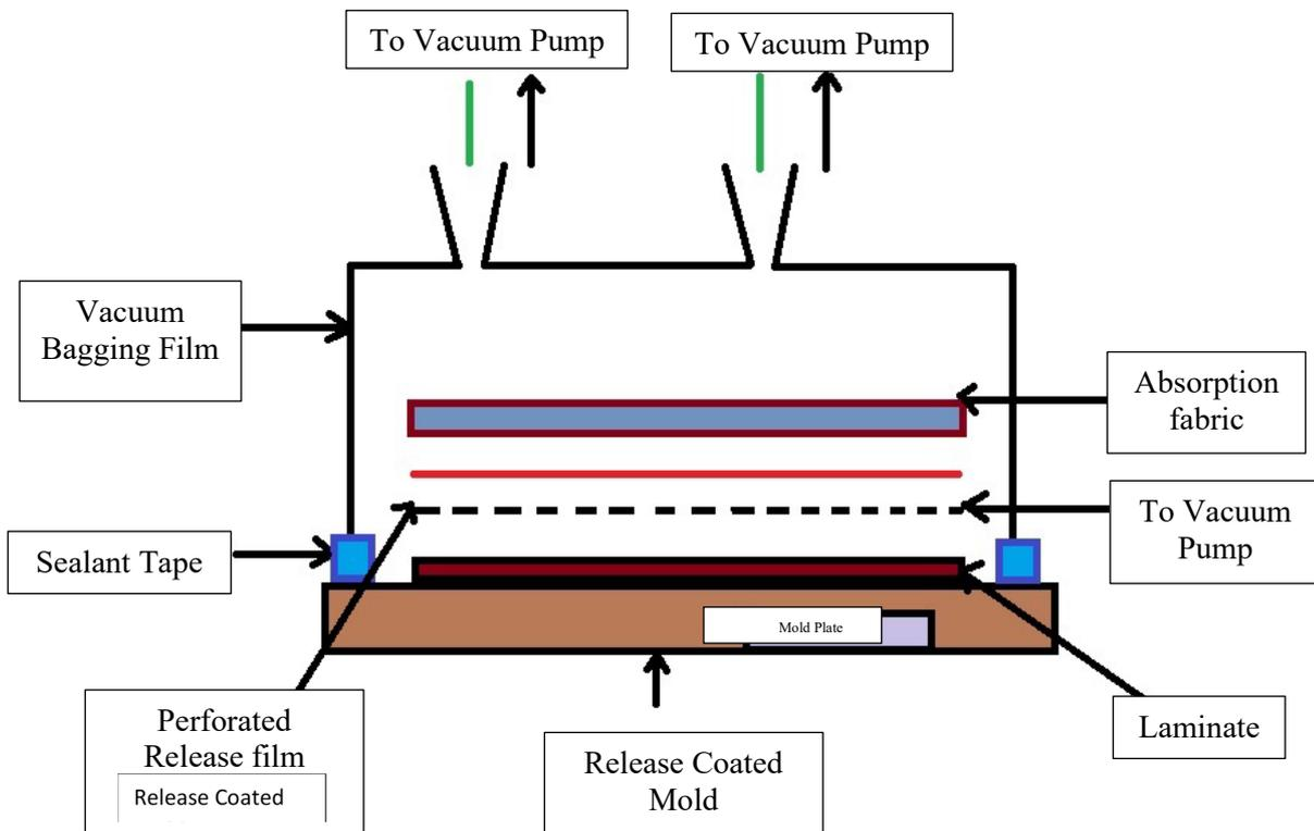
**Fig. 2.** Illustration of Vacuum Bag Molding Process.
