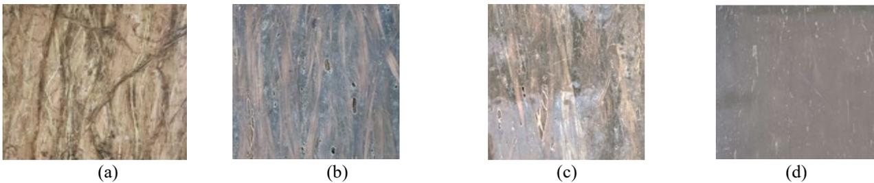
**Fig. 5.** The different fabricated samples of Titanium carbide nanoparticles reinforced kenaf-coir hybrid epoxy composite sample with (a) 0 wt.% of TiC (b) 3 wt.% of TiC (c) 4 wt.% of TiC (d) 5 wt.% of TiC
