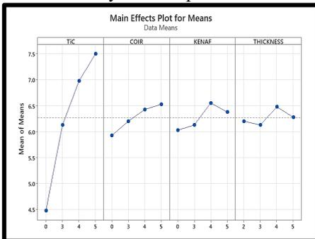
Fig. 12. Main effects plot of Flexural Modulus for TiC reinforced kenaf coir hybrid composite
