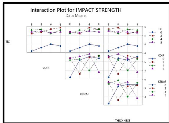
Fig. 17. Interaction Plot of Impact Strength for TiC reinforced kenaf coir hybrid composite.
