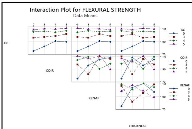
Fig. 16. Interaction Plot of Flexural Strength for TiC reinforced kenaf coir hybrid composite
