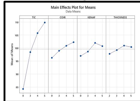
Fig. 11. Main effects Plot of Flexural Strength for TiC reinforced kenaf coir hybrid composite
