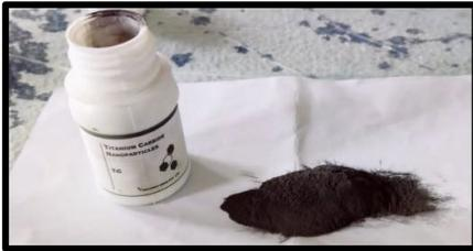
**Fig. 3.** Titanium Carbide Nanoparticle Powder
