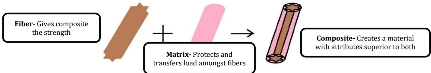
**Fig. 1.** Blend of matrix and fiber to develop a Composite
