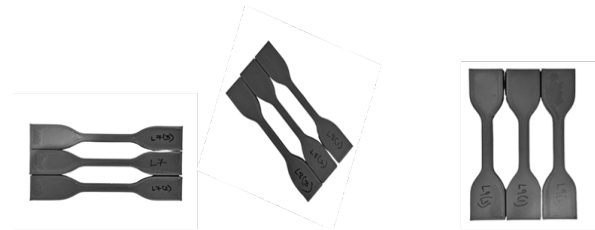
Fig. 4. L7, L8 and L9 Specimens printed at 0°, 45° and 90° after removing Support Structures
