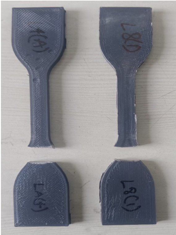
Fig. 6(a). Fractured tensile test specimens
