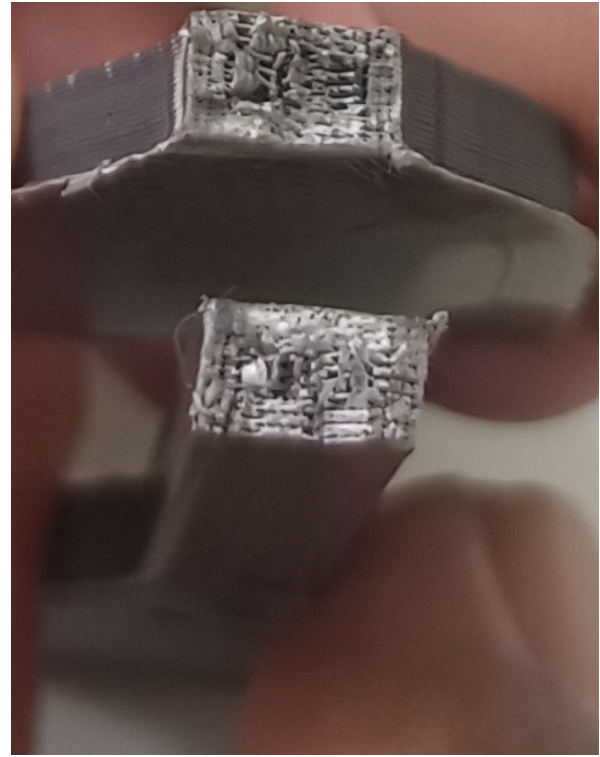
Fig. 6(b). Fractured surface of tensile test specimen
