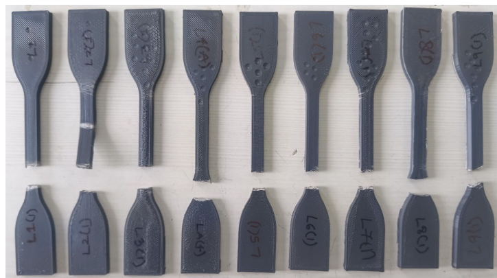
Fig. 5. Tensile test specimens after conducting tensile test on UTM.
