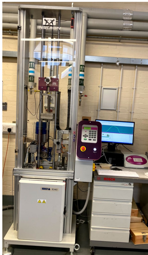
Fig. 1. CEAST 9340 drop weight impact machine developed by INSTRON® used in experimental tests
