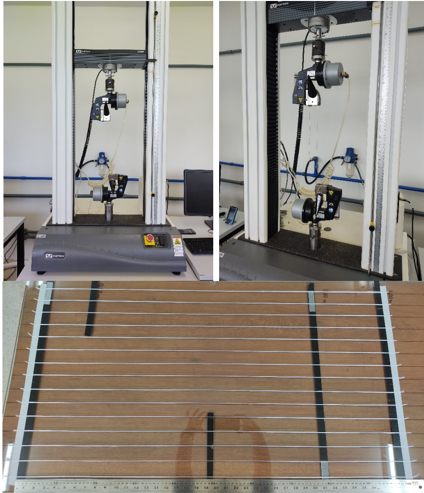
Fig. 1. Instron 3365 Equipment (left); Sample inside test machine (right); Sample preparation (below).
