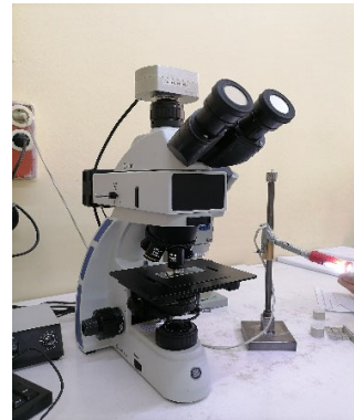
Fig. 1. instrument of indentation model “QNESS Q30 M” and visualisation “Euromex universal microscope of the type OXION”
