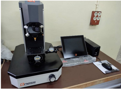
Fig. 1. instrument of indentation model “QNESS Q30 M” and visualisation “Euromex universal microscope of the type OXION”
