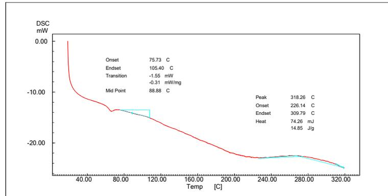
**Fig. 3.**  $T_g$  of the epoxy resin filled with 4 wt%,  $\text{Fe}_3\text{O}_4$  nanofillers
