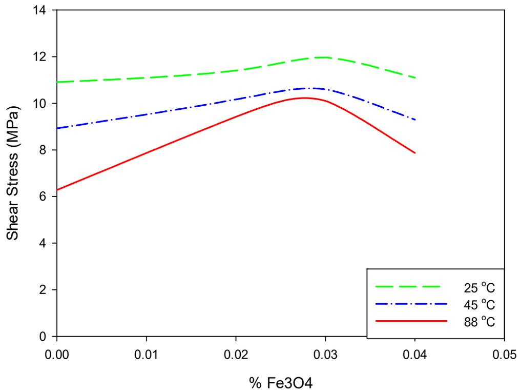
Fig. 13. Shear Strength of the Epoxy-Fe<sub>3</sub>O<sub>4</sub> composite with Fe<sub>3</sub>O<sub>4</sub> content
