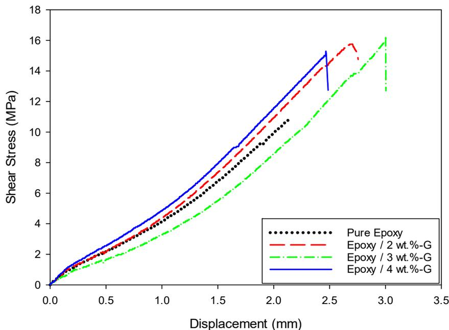
**Fig. 4.** Stress-Displacement curve of the Epoxy-Graphene composite with different weight fractions at 25°C.
