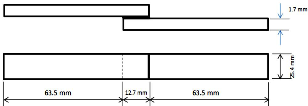
**Fig. 1.** Single-lap joint specimen dimension according to ASTM-D1002
