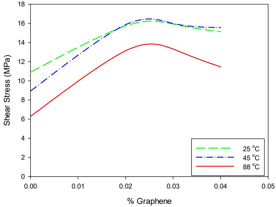
Fig. 12. Shear Stress of Epoxy-Graphene Composite with different weight fractions of G at different temperature tests
