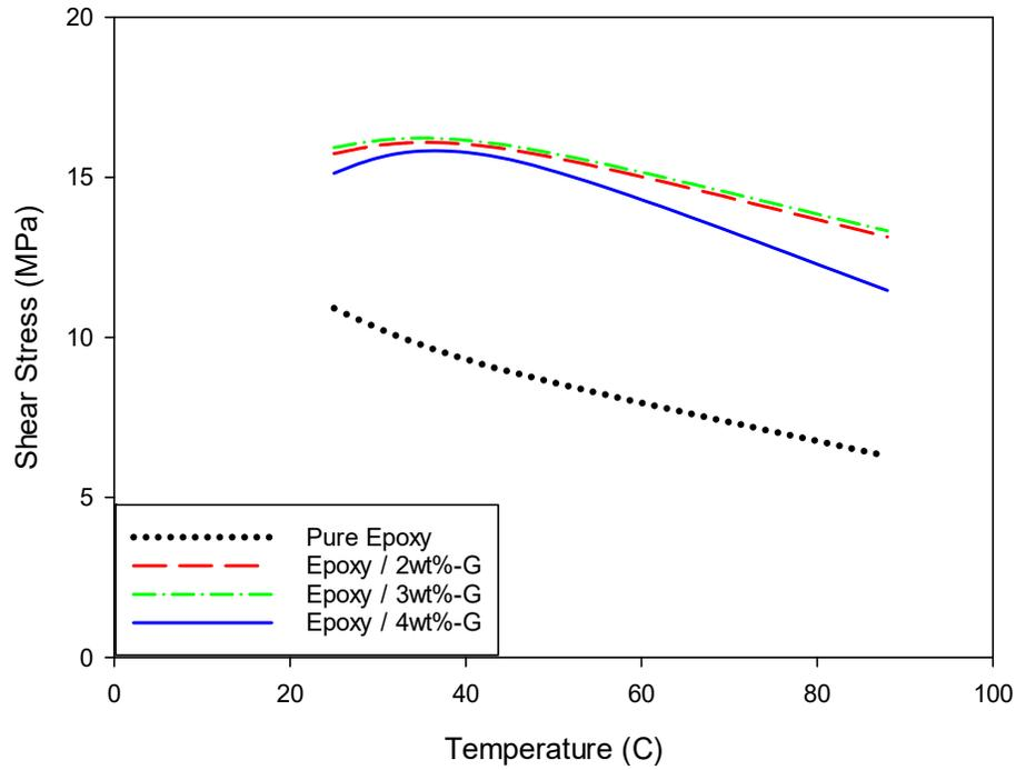
**Fig. 10.** Shear Strength of the Epoxy-Graphene Composite under various temperatures
