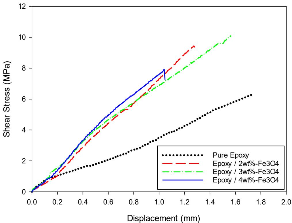
**Fig. 9.** Stress-Strain curve of the Epoxy-Fe<sub>3</sub>O<sub>4</sub> composite with different weight fractions of Fe<sub>3</sub>O<sub>4</sub> nanofillers at temperature test 88 °C.
