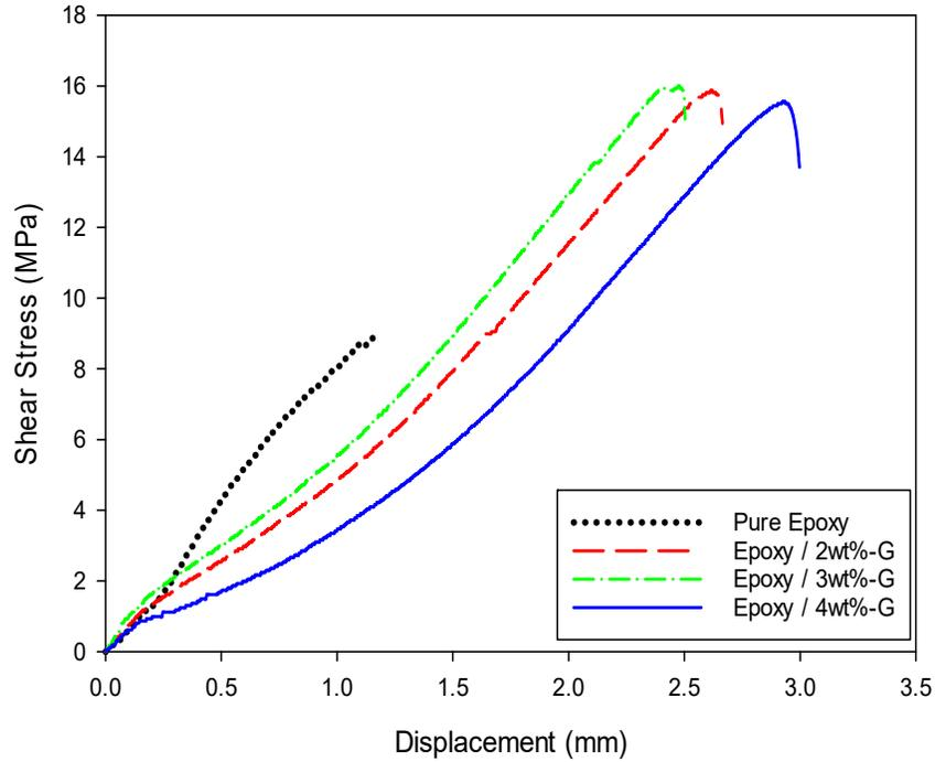
**Fig. 5.** Stress-Displacement curve of the Epoxy-Graphene composite with different weight fractions at 45°C.
