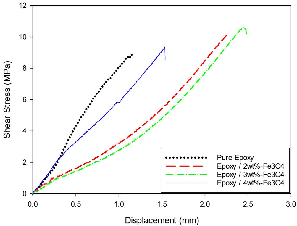
Fig. 8. Stress-Displacement curve of the Epoxy-Fe<sub>3</sub>O<sub>4</sub> composite with different weight fractions of Fe<sub>3</sub>O<sub>4</sub> nanofillers at 45 °C.
