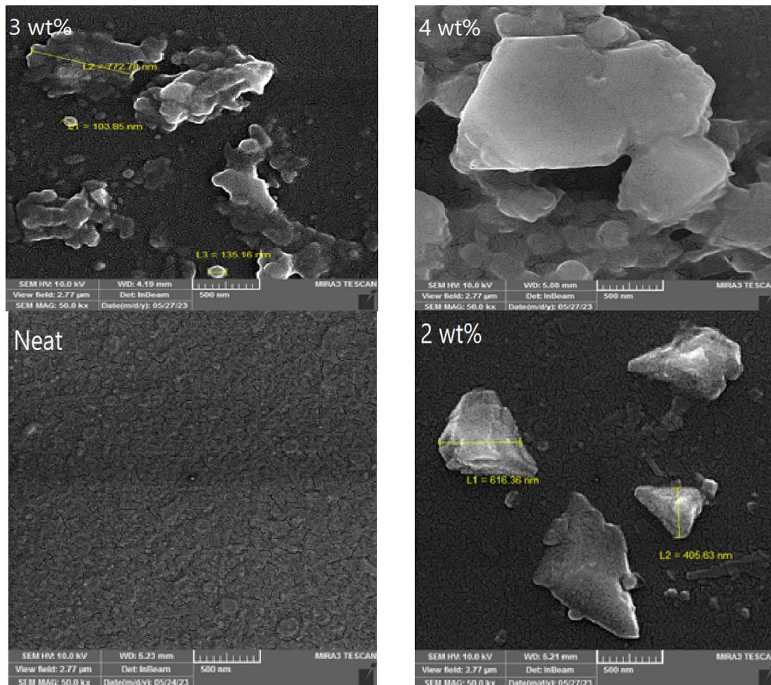
**Fig. 14.** The SEM micrographs of distribution of Graphene nanoplatelets nanofillers mixing with epoxy.
