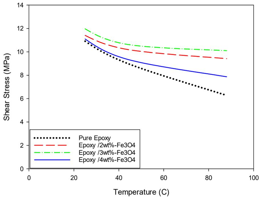
**Fig. 11.** Shear Strength of the Epoxy- $\text{Fe}_3\text{O}_4$  Composite under various temperatures
