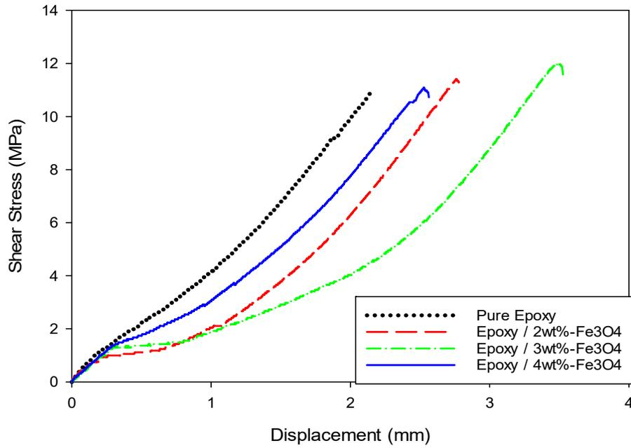
Fig. 7. Stress-Displacement curve of the Epoxy-Fe<sub>3</sub>O<sub>4</sub> composite with different weight fractions of Fe<sub>3</sub>O<sub>4</sub> nanofillers at 25 °C
