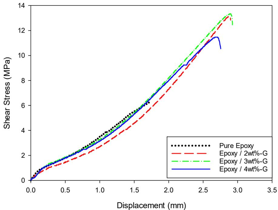
**Fig. 6.** Stress-Displacement curve of the Epoxy-Graphene composite with different weight fractions at 88°C.
