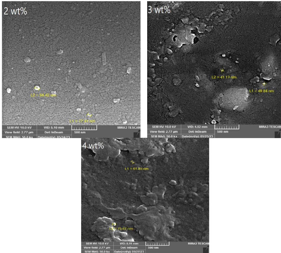
**Fig. 15.** The SEM micrographs of distribution of  $\text{Fe}_3\text{O}_4$  nanofillers mixing with epoxy.
