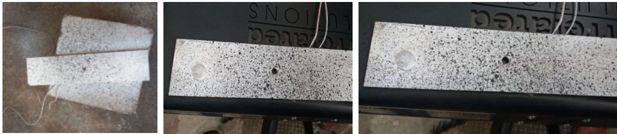
Fig. 2. Speckle image of Aluminium Specimen
