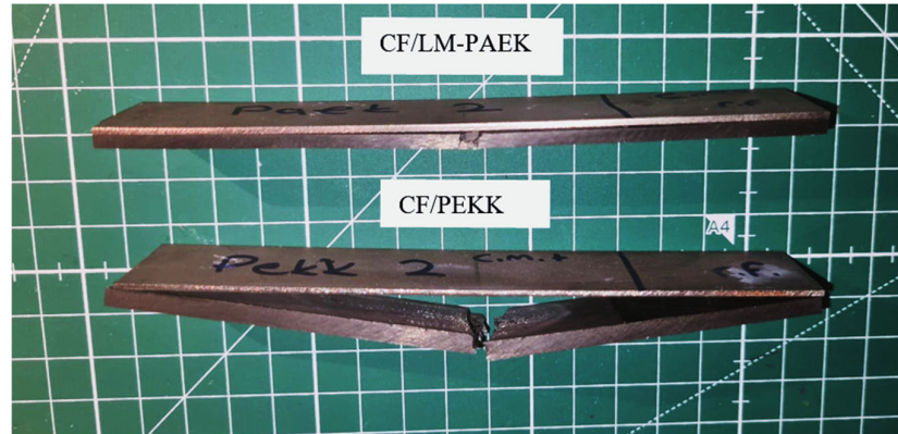
Fig. 5. The front view of the specimens after ENF test
