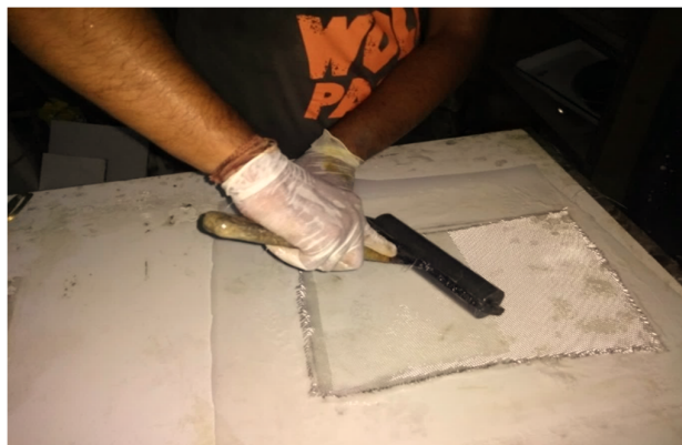
Fig. 1. Fabrication process using hand lay-up method
