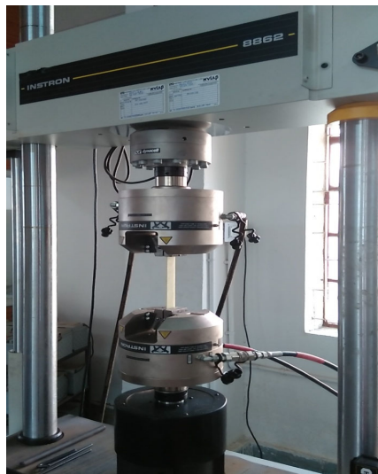
Fig. 2. Tension-tension fatigue test
