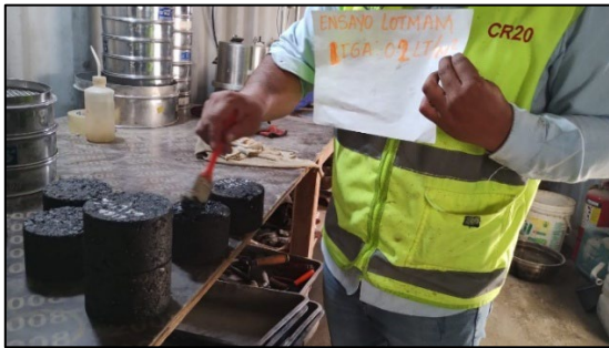
Fig. 3. Application of the ligator irrigation with 0.2 l/m 2
