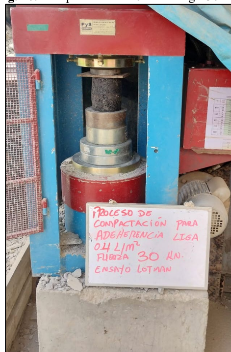
Fig. 12. Compaction Rate 0.4 l/m 2 kgf. 30 KN
