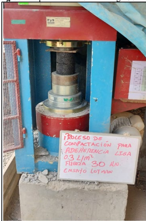
Fig. 11. Compaction Rate 0.3 l/m 2 kgf. 30 KN
