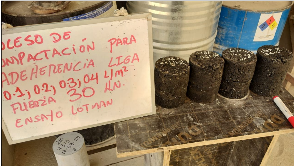
Fig. 13. Group of pastons enabled for the Lottman test
