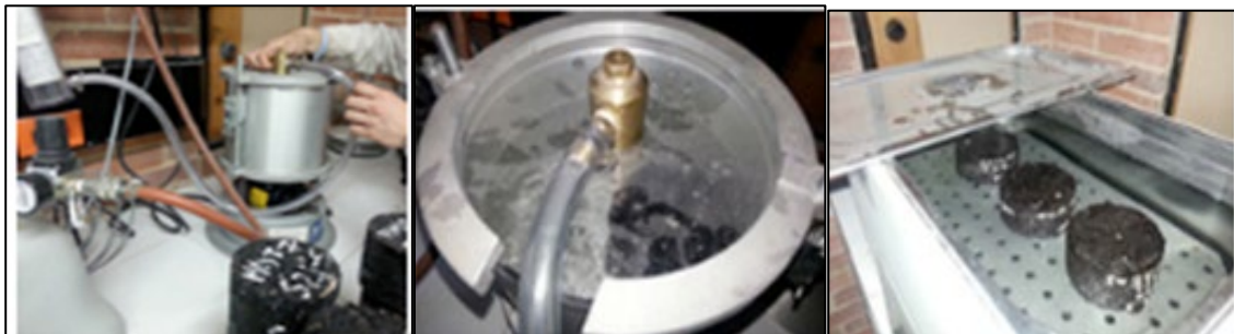
Fig. 15. Rice Test and Samples in the Bain-Marie to start with the Lottman rupture tests
