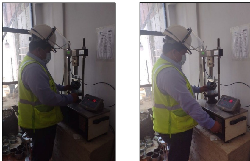
Fig. 16. Lottman test of conditioned briquette breakages with different league irrigation rates.
