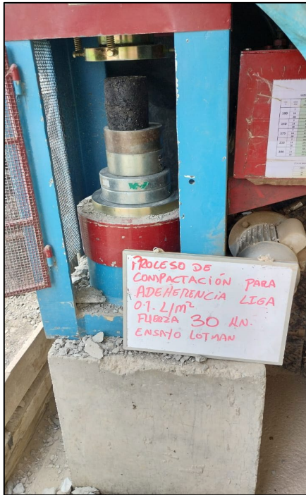
Fig. 9. Compaction Rate 0.1 l/m 2 kgf. 30 KN
