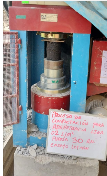
Fig. 10. Compaction Rate 0.2 l/m 2 kgf. 30 KN
