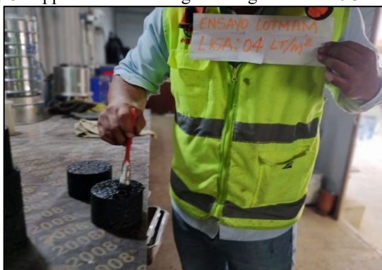
Fig. 7. Application of the ligator irrigation with 0.4 l/m 2
