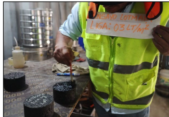
Fig. 5. Application of the ligator irrigation with 0.3 l/m 2
