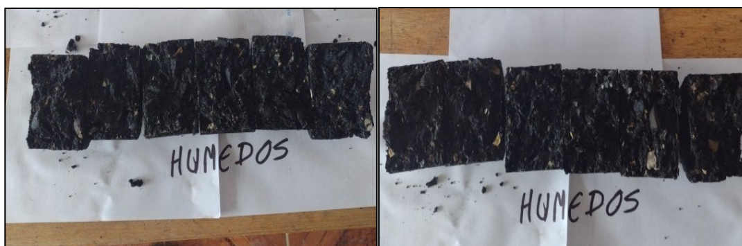
Fig. 17. Asphalt pastones carried out by the Lottman test
